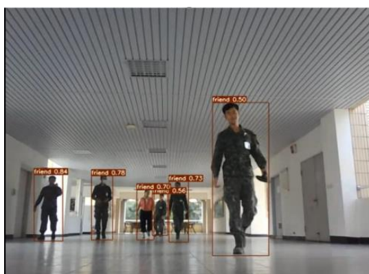
Figure 8: During long-range testing of individuals clad in camouflage attire, recognition remains viable
